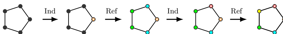
■ Figure 1 An illustration of the IR process. Individualization steps break symmetries or similarities (nodes marked with a cross are individualized). Refinement steps propagate this information.
