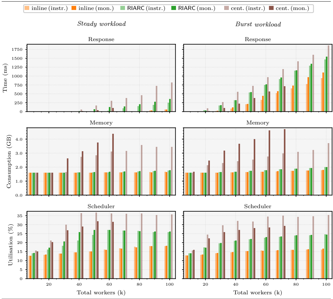
■ Figure 8 Instrumentation and RV monitoring overhead gap ( high workload, 100k workers).
