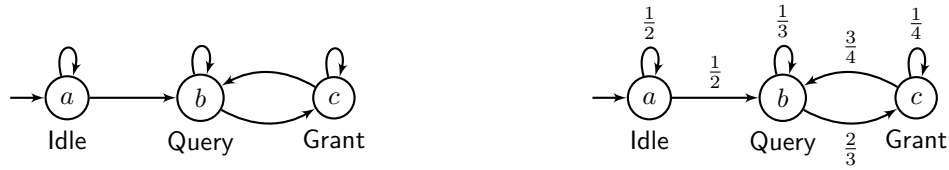
■ Figure 1 A protocol modeled as an LTS on the left, and as a probabilistic system on the right.
