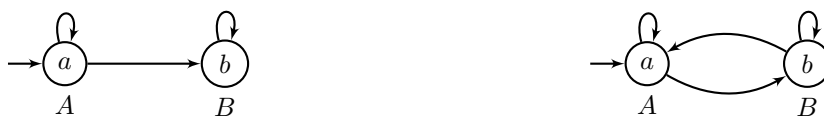
■ Figure 6 Two systems that satisfy F^\infty A \vee F^\infty B . The one on the left does not satisfy F_p^\infty A \vee F_p^\infty B unless its “initialization period” is ignored. The rightmost one does not satisfy it either ways.
