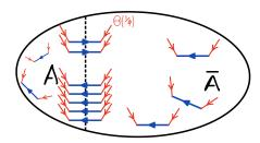
(a) In directed graphs, cuts are asymmetric. While  $(A, \bar{A})$  might be a sparse cut, the cut  $(\bar{A}, A)$  might contain many edges. A straightforward extension of [31] would inject  $2/\phi$  units of commodity to each endpoint of  $E_G(A, \bar{A}) \cup F$ . However, it is not clear with this approach how to bound the total amount of flow injected throughout the algorithm.
