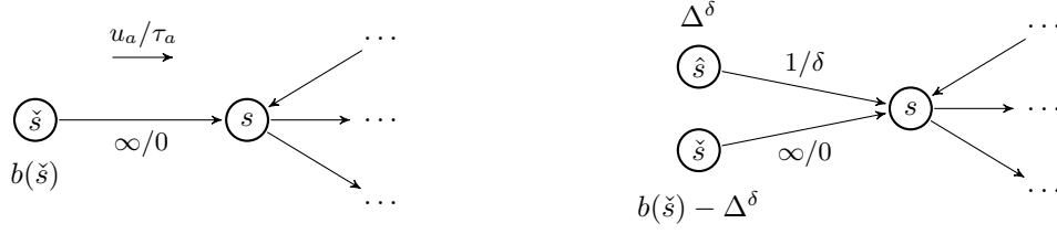
■ Figure 2 A dynamic transshipment instance (\mathcal{N}, b, T) after initialization with terminal \hat{s} (left) and the corresponding \delta -parametric instance (\mathcal{N}^\delta, b^\delta, T) for MINIMIZEDELTA (right).
