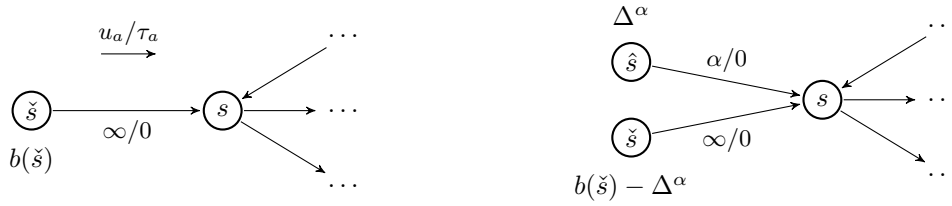
■ Figure 1 A dynamic transshipment instance (\mathcal{N}, b, T) after initialization with terminal \check{s} (left) and the corresponding \alpha -parametric instance (\mathcal{N}^\alpha, b^\alpha, T) for MAXIMIZEALPHA (right).
