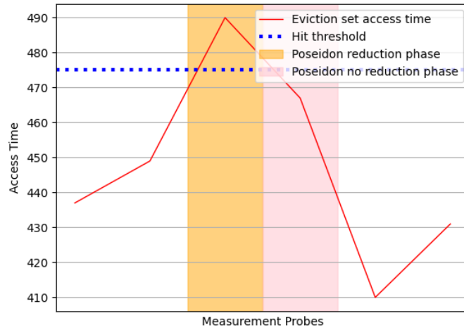
(b) Probe measurements of POSEIDON-GL hash function with P+P attack. In the orange phase, the round constant addition is followed by the modulo reduction operation. In the pink phase no such reduction is performed. We probe the eviction set contained in the cache-set where the reduction operation instruction also lies, giving slower probe time compared to the phase not executing the modulo reduction.
