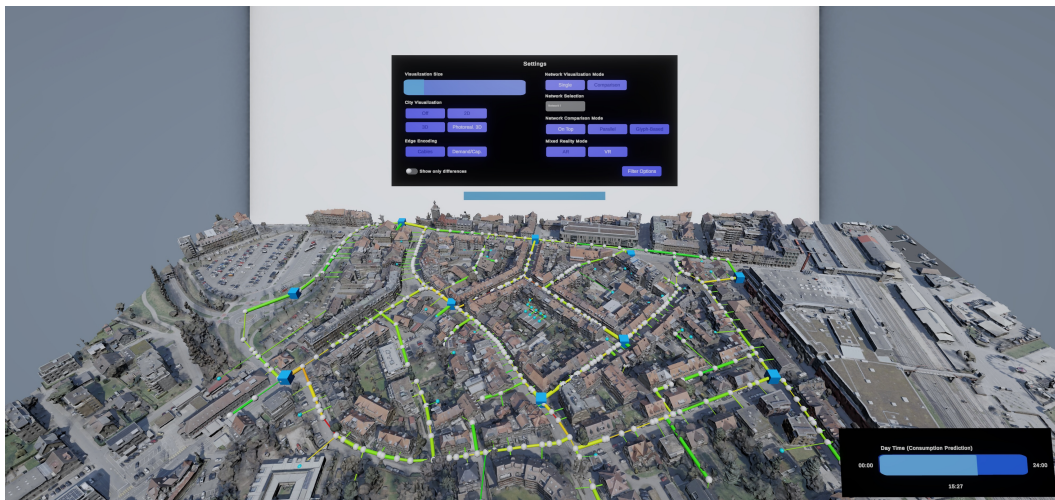
■ Figure 1 The EnMRgy system in the MR environment, consisting of the visual representation embedded in a 3D city model, a settings menu, and a slider to adjust the daytime used for demand simulation. Shown is a non-restricted version of an actual electricity distribution network.
