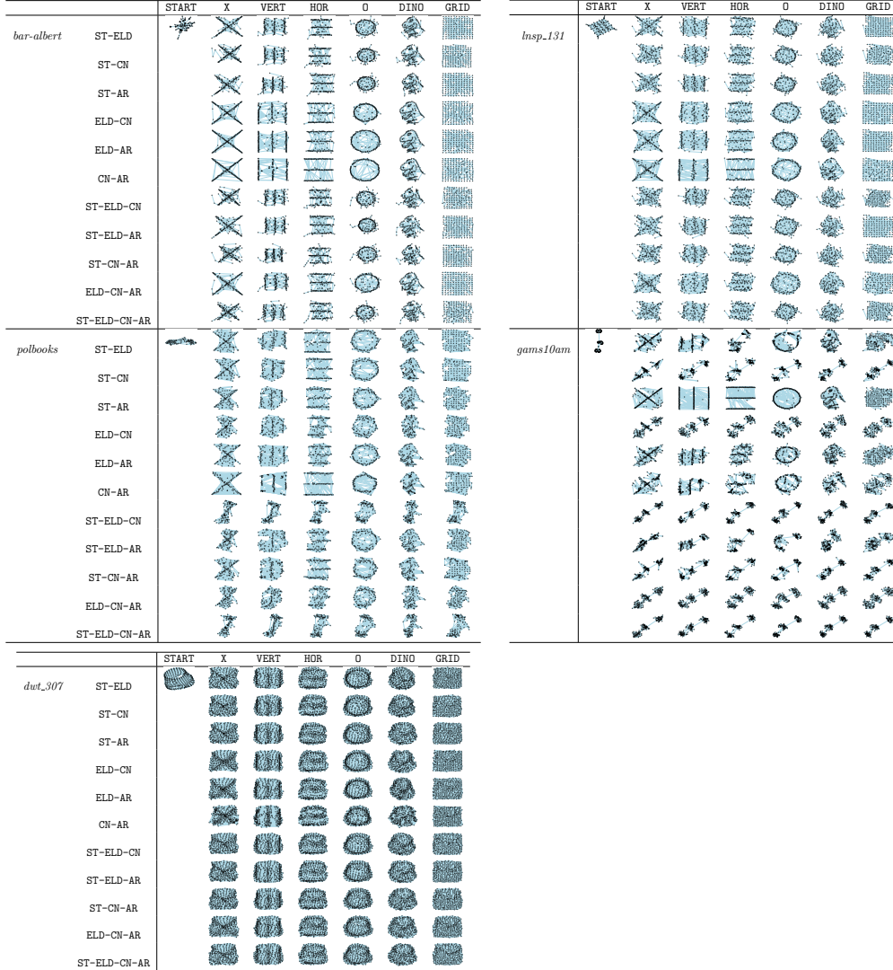
Figure 5 Collection of different graph drawings. The START column indicates the starting drawing of various graphs. The results of applying Alg. 1 to START to six target shapes ( X , VERT , HOR , O , DINO , GRID ) are shown in their respective columns. The rows indicate the metrics that have \pm\epsilon = 0.0025 for combinations of ST, ELD, AR and \pm\epsilon = \text{CN}(\Gamma) * 0.05 for CN.
