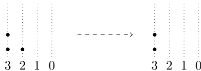
■ Figure 9 Shifting: size(BA_3^{2,3,3}) = size(BA_2^{3,3}) . In turn, BA_2^{3,3} can be computed by the Half Adder. Thus, BA_3^{2,3,3}(x_1, x_2, x_3) = (x_1, x_2 \oplus x_3, x_2 \wedge x_3) .
