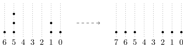
■ Figure 5 The function \text{BA}_7^{0,1,1,5,5,5,6}: \{0, 1\}^7 \rightarrow \{0, 1\}^6 replaces seven bits of significance (0, 1, 1, 5, 5, 5, 6) with six bits of significance (0, 1, 2, 5, 6, 7) .
