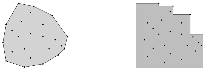
■ Figure 1 Examples of a convex hull (left) and the maxima (right) of a planar point set. We let N and H denote the number of input and output points, respectively.
