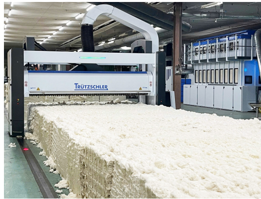
■ Figure 1 Photograph of the cotton bale, mixing table, and cotton-feeding head of the blending machine at the company under study.
