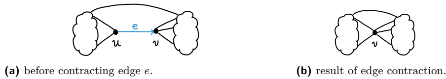
■ Figure 3 Edge contraction of edge e identifies its source and target vertices.
