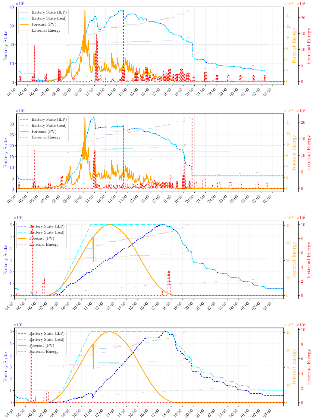
■ Figure 12 Illustration of ILP solution for RA with \lambda = 0.94 for operational day March 13 in year 2020 (upper half) and in year 2022 (lower half). In each half, the upper and lower plot corresponds to flexibility 0 and 3, respectively. The total required external energies for flexibility 0 and 3 are 84210 respectively 75497 for 2020, and 9876 respectively 5275 for 2022. Jobs are depicted as colored stripes, each at its unique \gamma -value (corresponding to the job's index). We present both battery states: those computed by the ILP, and the “real” ones in the sense of when the jobs are scheduled according to the ILP solution.
