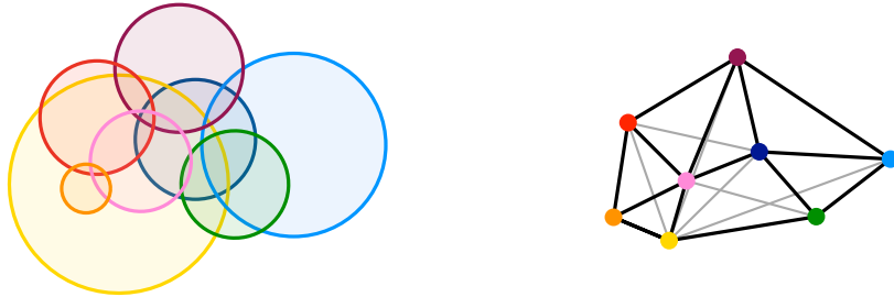
■ Figure 1 A set of disks \mathcal{S} (left) and the corresponding disk graph \mathcal{D}(\mathcal{S}) (right) that includes both the thick black and the thin grey edges. The thick black edges form a (1 + \varepsilon) -spanner for \varepsilon = 3/4 .
