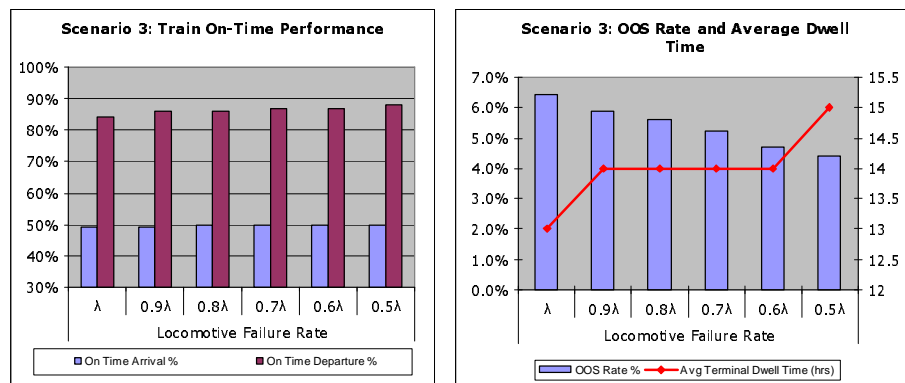
Fig. 12. On-Time Train Performance, Out-Of-Service Rate and Average Terminal Dwell Time for Different Values of Locomotive Failure Rates.
