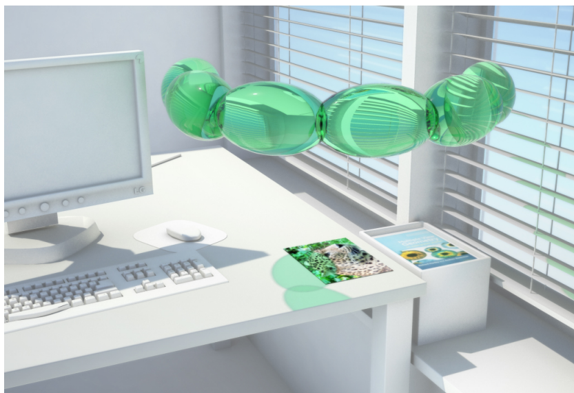
■ Figure 4 Modeling the camera pose prior probability by mixtures of Gaussians. For simplicity, only the translation uncertainty is visualized (green ellipsoids). A real pose prior probability would normally consist of a 6D covariance. The mean values \mathbf{x}_Q hereby specify the position, the covariances \Sigma_Q the shape of the ellipsoids.
