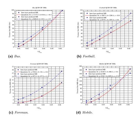
**Figure 1** Relationship between average number of texture bits and Q<sub>step</sub> for both inter-layer coding and non-inter-layer coding. Points are actual data; curves are fitted to the data.
