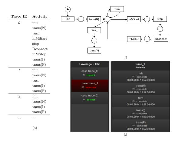
**Figure 1** (a) Generated traces from an Infusion Pump, (b) Discovered Model, (c) Verifying property.
