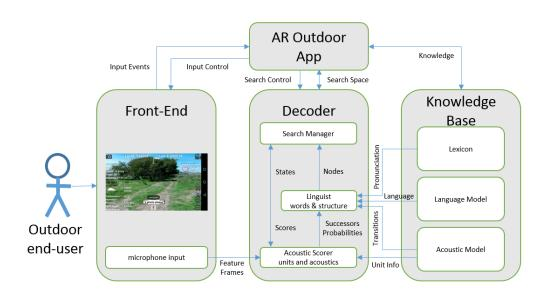
**Figure 1** Sphinx System Architecture [12, 13].
