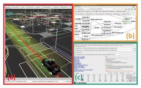
Figure 2 Screenshot of co-simulation using IDF-Autoware: (a)RViz displaying Autoware status, (b) the rqt\_graph\_autoware, and (c) the Runtime Manager for IDF-Autoware.
