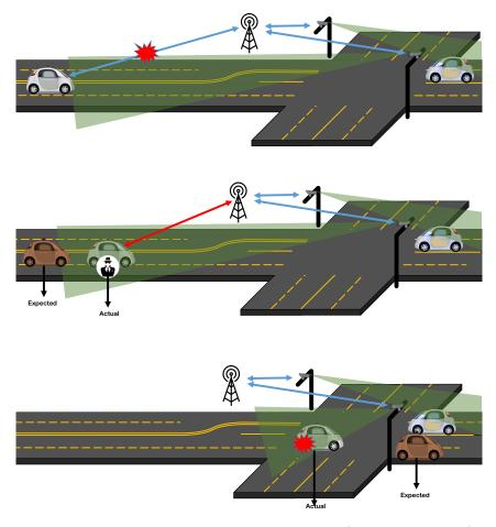
**Figure 7** Three beneficial scenarios of the Detection System (from top to bottom): when the vehicle's communication systems are malfunctioning, when an attacker claims there is a vehicle nearing the intersection when there is not, and when there is a discrepancy between the connected data and environmental detection data.
