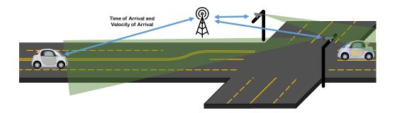
**Figure 3** RIM Robust has a surveillance Detection system that monitors the position of vehicles and reports it to the IM.
