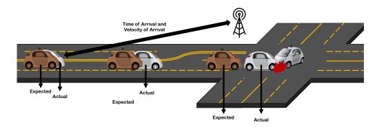
**Figure 1** RIM Algorithm: A car will communicate with the IM to get a Time of Arrival (TOA) and Velocity of Arrival (VOA). However, it may not be able to meet the TOA and VOA and can cause an accident.
