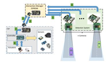
**Figure 2** The IM, Detection System and vehicle interact with each other in five steps to verify the car data using the environmental sensing data.
