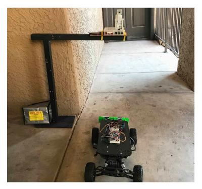
**Figure 4** At one corner of the intersection, you can see one of the four subsystems of the Detection System mounted on top of the wooden infrastructure with a TRAXXAS RC Car about to drive underneath.
