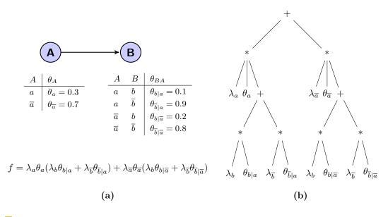
**Figure 3** (a) A Bayesian network with a multilinear function. (b) The corresponding arithmetic circuit.
