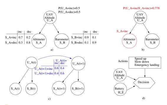
**Figure 1** BN principle and DN example: a) BN example, b) Inference illustration, c) Dynamic BN, d) DN example.
