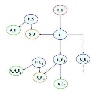
**Figure 4** FMEA\_HM pattern for BN where the  $S\_U$ ,  $S\_Ei$  nodes represent the sensor nodes of either a hardware or a software monitor, the nodes U,  $U\_Ei$  are the internal states possibly affected by an error Ei, the  $H\_U$  node represents the health of the system,  $H\_S$  and  $H\_Ei$  nodes represent the health of the sensor, and the  $A\_H$ ,  $A\_H\_Ei$  are the appearance contexts.
