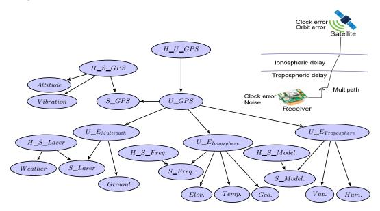
**Figure 6** GPS potential errors and BN description.
