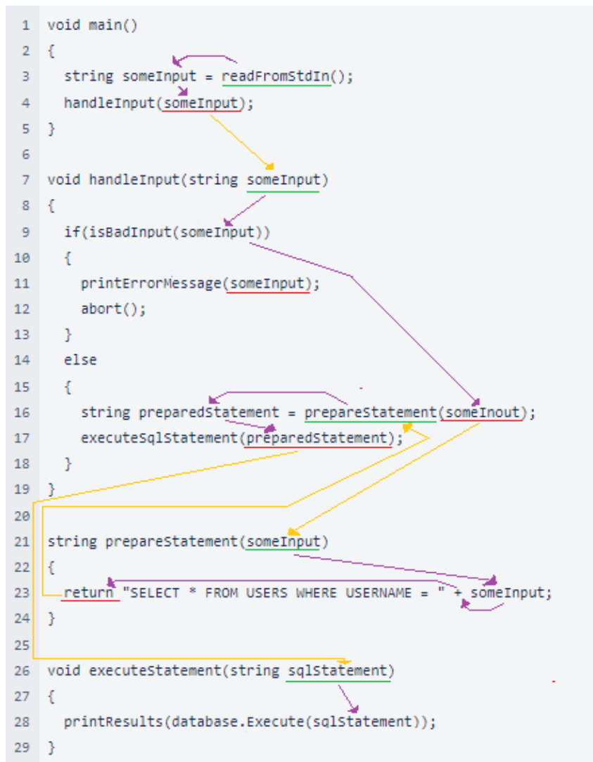
■ Figure 2 Flows inside functions: purple arrows are paths along lines of code while yellow arrows are just empty edges.
