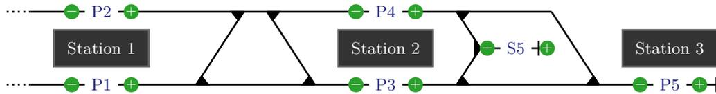
■ **Figure 2** A schematic plan of the infrastructure with labeled ends at infrastructure points.
