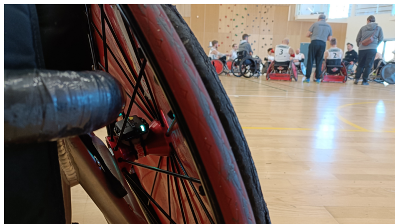
■ Figure 6 Figure 6: Sensor placement in the wheel for capturing performance data.
