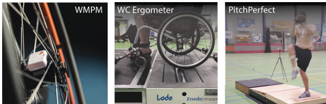
■ Figure 1 Figure 1: The Wheelchair Mobility Performance Monitor (WMPM) is an Inertial Measurement Unit (IMU)-based field solution to measure the overall on-court power demands during training and competition. The Esseda wheelchair (WC) ergometer is a high- resolution measurement tool to analyse how the power is optimally delivered by an athlete under standardized repeatable conditions in their personal sports. Third, the PitchPerfect system is also an IMU-based tool, originally developed for pitching in baseball but also employable in wheelchair sports, especially wheelchair tennis, to provide coaches and athletes feedback on motion timing and power production through the kinetic chain in throwing and hitting.
