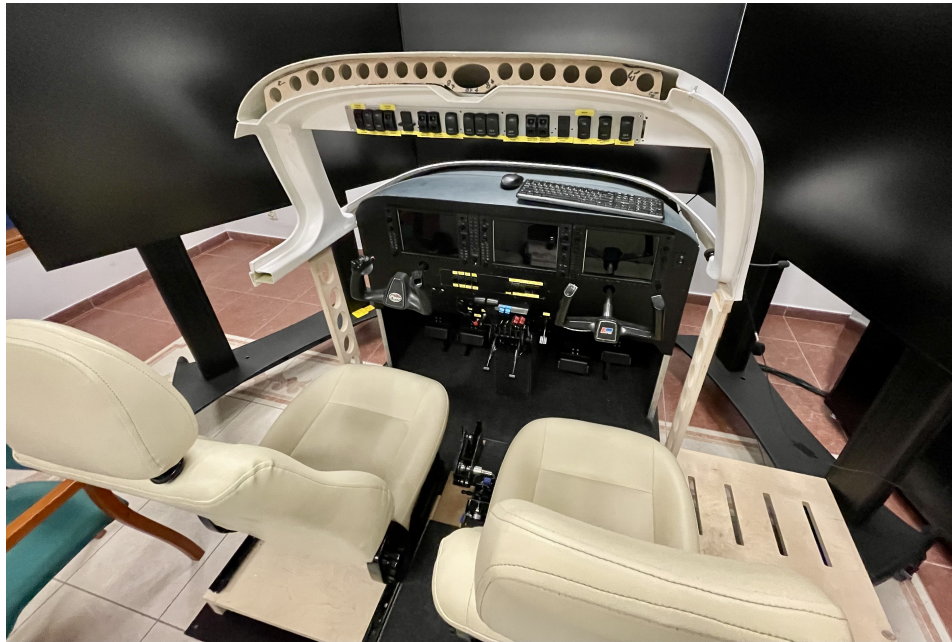
■ Figure 3 Flight and Navigation Procedures Trainer certified for single- and multi-engine aircraft procedures training. Source: own resources.
