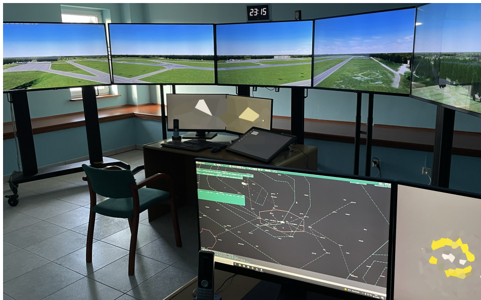
■ Figure 4 A certified 180-degree view tower simulator for ATCO training. In the foreground, a management station where the instructor can monitor performance in real time and interact with the simulation by initiating non-standard or emergency situations. Source: own resources.
