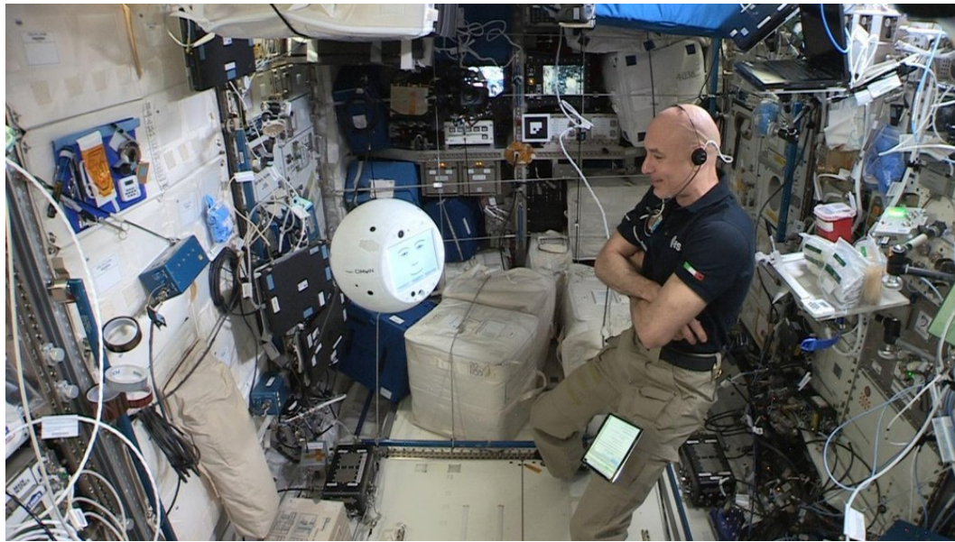
■ Figure 1 CIMON, an early example of an intelligent personal assistant deployed aboard the International Space Station. It served as a proof of concept for voice interaction in microgravity but was limited by its reliance on narrow AI and Earth-based processing.
