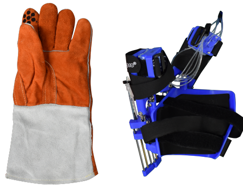
■ Figure 7 The benchmark heavy work glove with markings for input positions on the index finger (left), and the two-fingered human-side interface (right) used for testing the sensitivity to motion and positional pressure.
