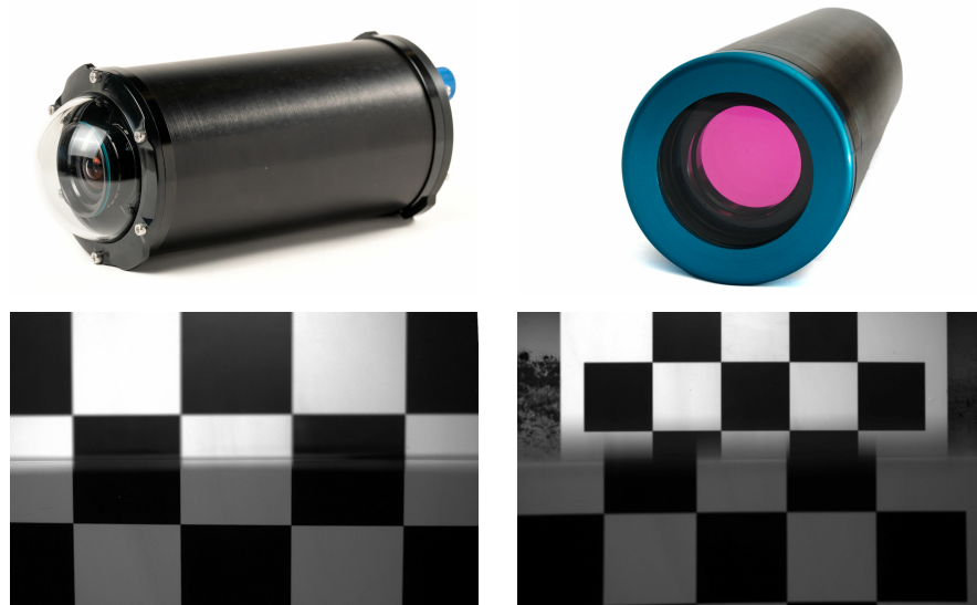
■ Figure 6 Dome port (above left) and flat port (above right) underwater camera. Below are two example images with the dome port (below left) and flat port (below right) partially submerged in water. The top half of the image is in air while the bottom half is in water.
