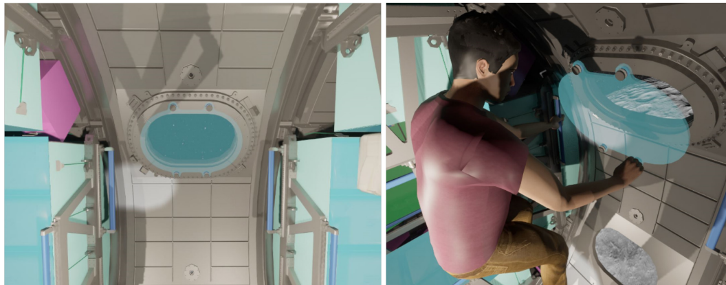
■ Figure 6 Scratch pane design concept under evaluation in ERM/Esprit module in Windows bay – virtual scenario with 99th mannequin simulating the neutral posture in 0g environment.
