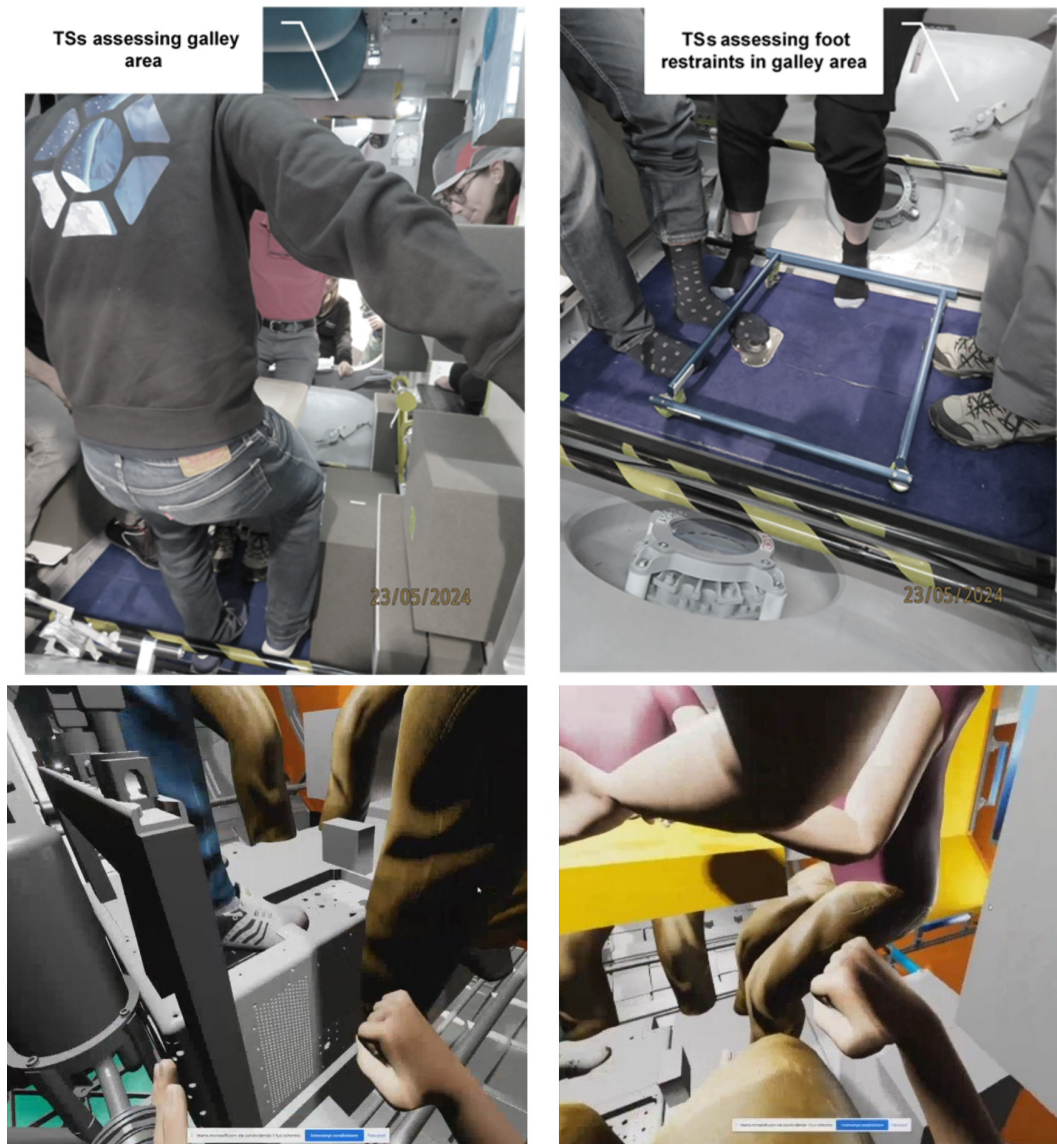
■ Figure 5 Comparison between physical (up) and virtual (down) environments where crew members and engineering users simulated the tasks the Galley area and a table concept to evaluate the feasibility to accommodate four crew of 99th percentiles for dinning together.
