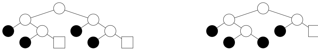
■ Figure 4 Examples for Lemma 13 with the binary distribution \mathbf{w} = (0, 2, 2) , where two binary trees exist, which can be complemented by adding dummy leaves. The left tree and the right tree can be complemented by the vectors (0, 0, 2) and (0, 1, 0) to full binary trees, respectively. Black nodes are leaves, and dummy nodes are rectangles.
