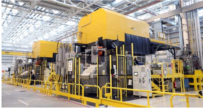
■ Figure 1 Aluminum die-casting machine.
