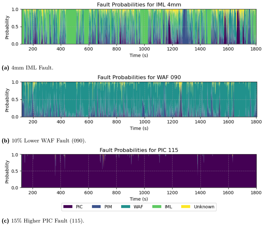
Figure 7 Stacked isolation probabilities over time for 4mm IML fault (a), 10% lower WAF fault (b), and 15% higher PIC fault (c). The fault probabilities are averaged over the last 20 predictions, starting after the fault occurs. The stacked bars have a fixed order, so the probability is denoted by the size of the bar at each time, not its proximity to the top of the y-axis.
