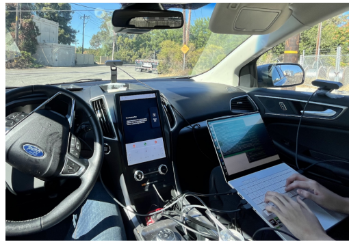
(b) Interior view showing the mounted camera and local laptop server.
