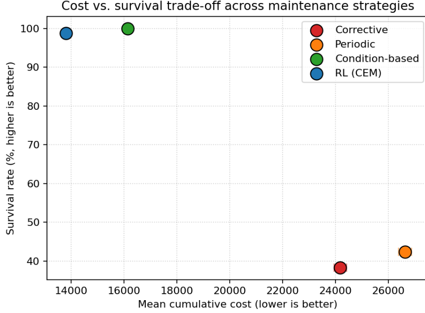
■ Figure 6 Cost–survival trade-off across the four strategies. The CEM policy strictly dominates the corrective and periodic baselines, and forms a Pareto frontier with the condition-based heuristic.
