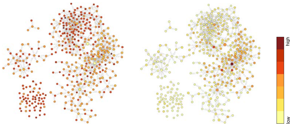
■ Figure 4 \epsilon -Machine of the delta wing using different color codings: (left) local statistical complexity of causal state and (right) number of edges per node.
