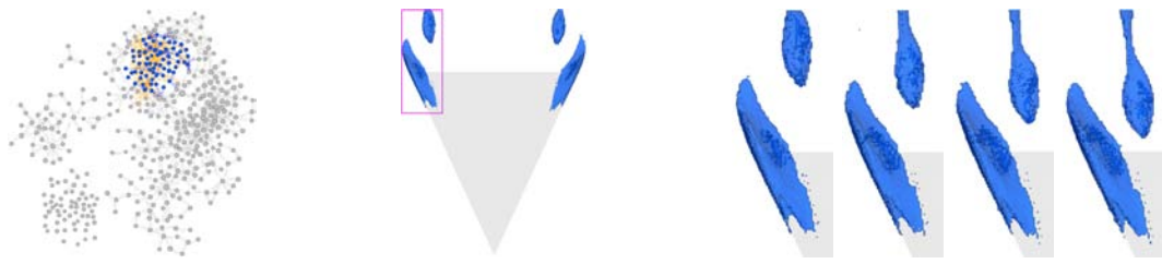
■ Figure 3 Evolution of the recirculating bubble in the delta wing data set: (left) \epsilon -machine; Selected nodes are colored in blue. (center) Corresponding positions in time step 650. The pink frame indicates the area of the closeup. (right) Physical positions with corresponding causal states in time steps 650, 670, 690, and 710.
