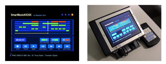
**Figure 4** SmartMusicKIOSK screen display. This is a music listening station with a chorus-search function. The lower window presents the playback operation buttons and the upper window provides a visual representation of a song's contents. A user can actively listen to various parts of a song while moving back and forth as desired on the visualized song structure (the "music map" in the upper window).
