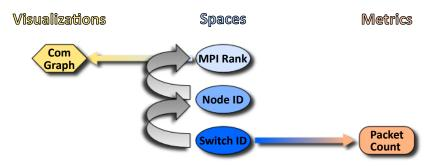
**Figure 4** A more complex context example of a communication graph operating on MPI ranks that shows network packets collected on a per network switch bases. The count is first projected to node ids according to the hardware configuration and subsequently to MPI ranks via the node mapping file stored at runtime.
