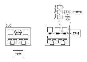
**Figure 1** An encryption and decryption unit at each core can help with better separation of cores.
