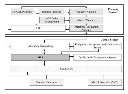
**Figure 1** Planning and Control System of a Semiconductor Supply Chain (adapted from [2]).
