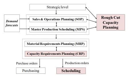
**Figure 2** Capacity planning in the planning and scheduling hierarchy.
