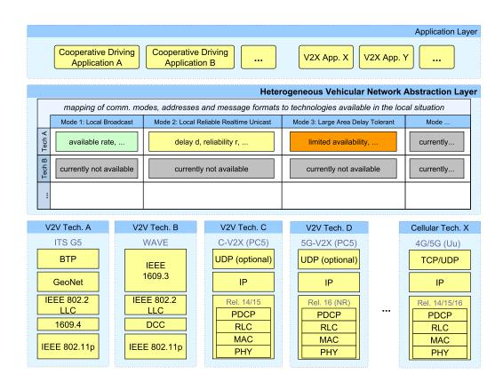
**Figure 2** Example illustrating the realization of a vehicular networking architecture implementing a heterogeneous vehicular network abstraction layer.
