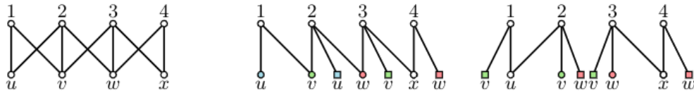
■ Figure 3 (a) A graph instance G ; (b) an optimal solution with three splits, involving three different vertices; (c) an optimal solution with two split vertices (but with more vertices in total).
