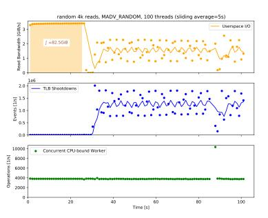
**Figure 1** Random 4K Reads from Memory-Mapped Device. Benchmark was executed on a AMD EPYC 7713 64-Core Processor with 512 GiB RAM
