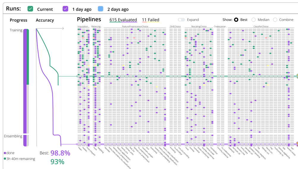
■ Figure 4 Our sketched visual interface to visualize AutoML/DS systems. An ongoing Auto-sklearn optimization is visualized in green. Additional past runs can be selected at the top for comparison. The table on the right shows the best performing configurations in the specific time segment.
