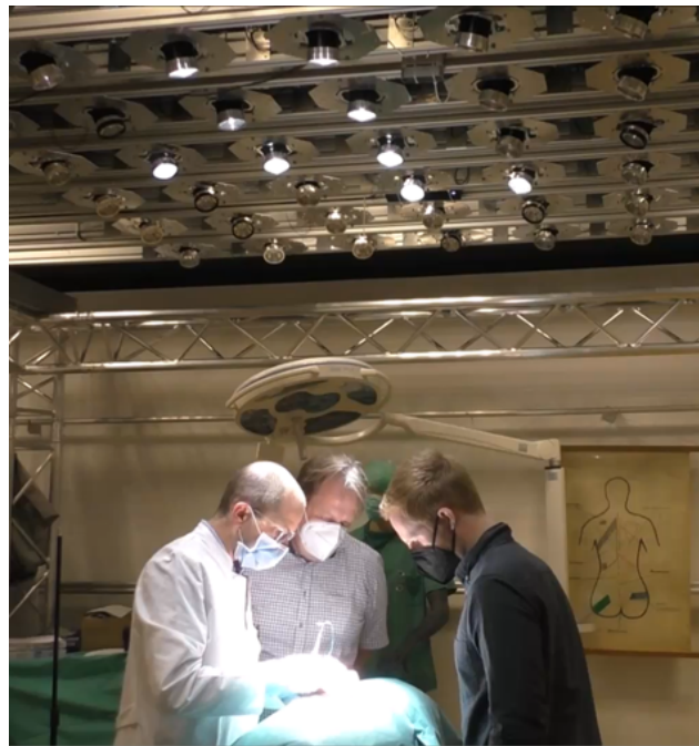
■ Figure 3 Photo of the demonstrator for a new operating room lighting system. The prototype will be installed in one of the new operating rooms at Pius-Hospital this year.
