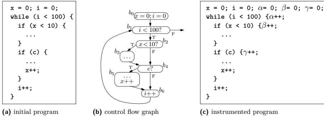
■ **Figure 1** Instrumenting an example program with counters.
