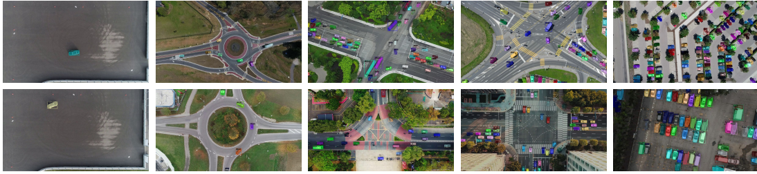
■ Figure 3 Detection examples: The left column depicts examples from the experiments performed on the test track. Other images are taken on roads, partly from publicly available sources [59, 44]. The masks, depicted with random colors, are used to compute the location, size and orientation of the smallest rectangle containing all mask pixels of the detected object. Note, the non-rotated bounding boxes would be the final output of typical object detectors without the segmentations masks.
