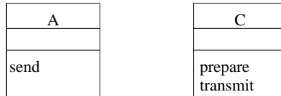
Fig. 3. Model transformation splitting an operation into two
